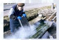
Katsushiro places the bamboo in boiling water to which he has added caustic soda, thus removing the bamboo's oil. Doing this and then drying the bamboo will make it last a long time.
